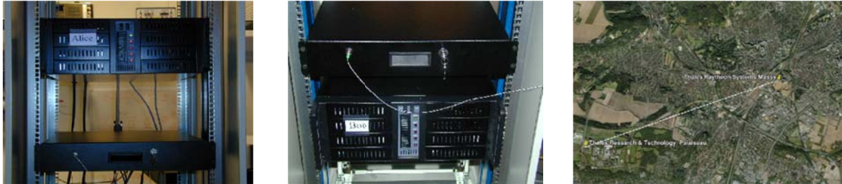
Figure 1: Prototype for quantum key distribution with continuous variables. The system was then tested during six months over a distance of 17.7km, and an improved version reached a distance of 80 km.
